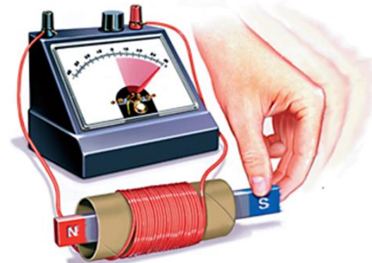
c A greater electric current is induced if you add more loops of wire. This magnet is moving at the same speed as the magnet in b .
